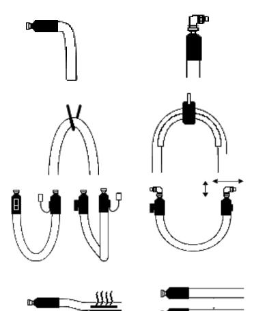
Narrow diameter causes the hose and heating cables to break. It should be shaped in the widest possible shape. Avoid sharp bending the hose, use angled and straight connection unions.
