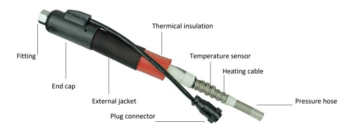
Heating hoses are designed and manufactured for the transfer of certain hot melt substances and gases. It keeps the temperature constant at desired values between melter and application head.
